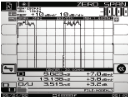
Zero span/time domain expert mode, showing the TDMA bursty return path cable modem power ramp of 3.5 ms
