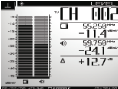
The single-channel level display shows both video and audio levels (either single or dual sound/ NICAM) and the difference between the two
