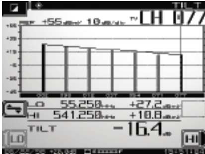
Tilt mode performs automatic tilt calculations between any two of nine designated carriers
