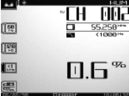
In-service "HUM" (PAL and NTSC compatible)
