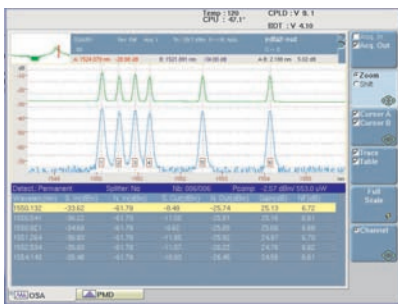
EDFA test application
