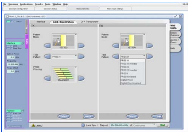
Unframed 10x10.3G BERT pattern configuration screen
