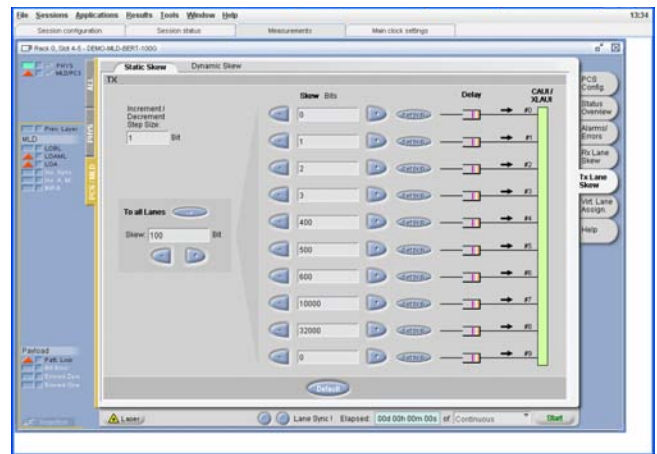
Lane Skew generation screen. Allows injection of static skew into each of the physical lanes.
