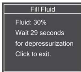
Step 4 Ensure that depressurization is completed.
