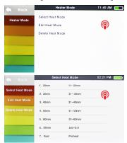
1 Enter "edit heat mode" menu via clicking "edit heat mode" in the interface of "Heater Mode"
