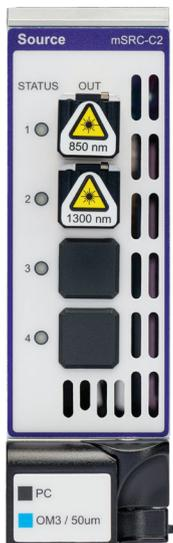
VIAVI offers a multiplexed and individual output low power LED as part of the general-purpose light sources (mSRC) in the MAP portfolio. The LEDs are offered at the common multimode wavelengths of 850nm and 1300nm. LED sources emit incoherent broadband light.
