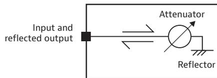
The MAP backreflector uses the VIAVI linear attenuator prism and high reflectivity mirror to precisely control the level of RL.
