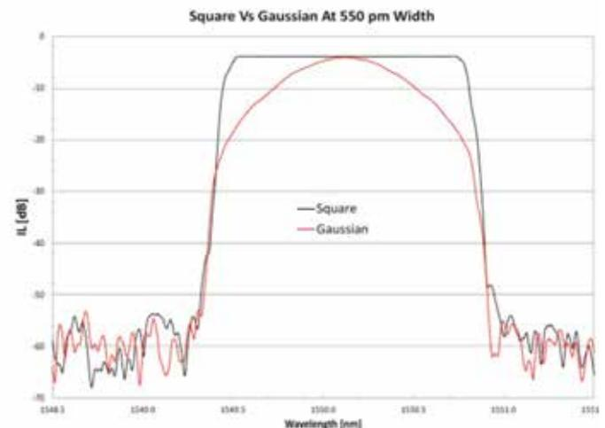
Figure 6 – Square and Gaussian filter using the mTFX
