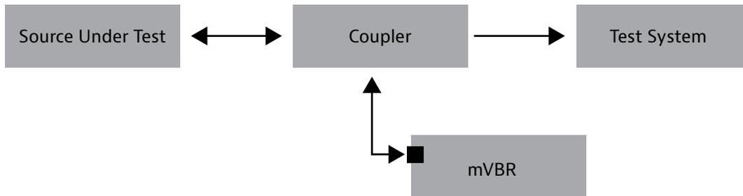
Figure 1 - Test configuration - mVBR cassette and external coupler
