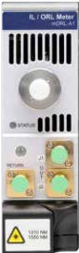
One slot single mode module contains up to four sources (1310, 1490, 1550, 1625 nm), and integrated power meter, and an optional 2x2 optical switch for automated bidirectional testing.
