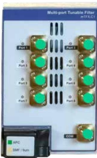
Get the right wavelengths to the right test port with the right power—quickly. Flexibly isolate, groom, manage, and route any wavelength or group of wavelengths with a simple, intuitive GUI and/or SCPI based remote commands. The mTFX-C1 is a modular instrument and can be directly managed from your PC-based automation system. It eliminates the need to re-purpose optical network technology or use complex libraries with specialized interface cards.
