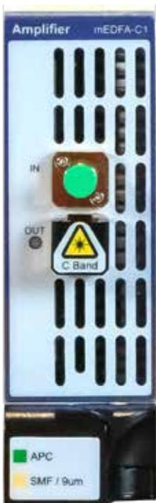
MAP Erbium-Doped Fiber Amplifier (mEDFA) Modules combine the optical performance of the traditional VIAVI benchtop models with the flexibility and modularity of the MAP series. The variants of the EDFA target diverse applications such as amplifier emulation, OSNR (optical signal-to-noise ratio) experiments, and network compliance tests.
