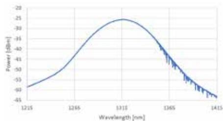
Figure 2: 1310nm SLED Spectral Width
