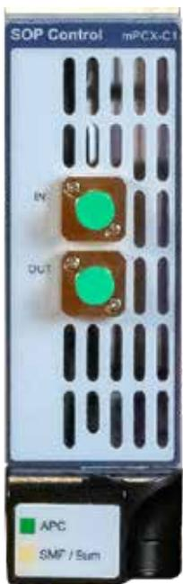
At its core, the mPCX-C1 cascades eight quarter wave-plates. Based on Lithium-Niobate, the electro-optic wave-plates have the response time required by the most demanding polarization management applications. These wave-plates can be rotated at high speed and are reset-free (endlessly rotatable) to control the state of polarization (SOP).
