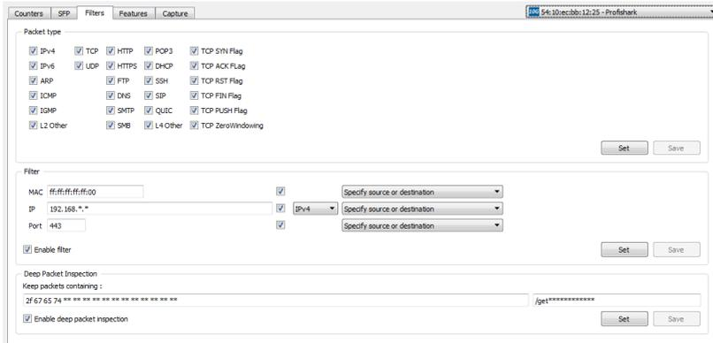
In the example above, the ProfiShark 10G has been set to capture only packets originating from or destined to any MAC address ending with 00, originating from or destined to any IPv4 address starting with 192.168, using port 443 for either incoming or outgoing traffic, and carrying matching DPI strings in their payload. The *Packet type* filter tells the ProfiShark which types of packets should be included in or excluded from the capture.
