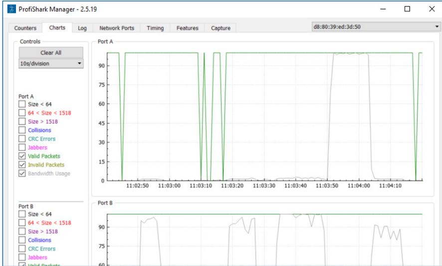
Depending on the type of packets or events selected in the left side of the screen, the statistical data is plotted accordingly for either port A or B. Refresh rate can also be selected using the drop-down list on the top left, further tuning the displayed information.
