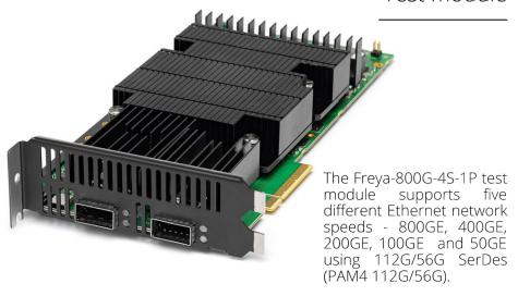
This flexibility is provided via two physical transceiver cages – one supporting QSFP-DD800 compatible transceivers, and the other supporting QSFP112 compatible transceivers.
