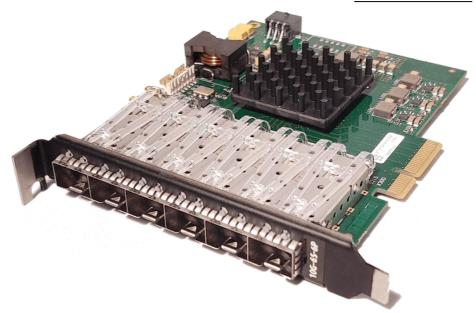
All 6 ports on the Odin-10G-6S-6P can be quickly configured to individually test any of the 6 speeds – 10M, 100M, 1GE, 2.5GE, 5GE 10GE.
